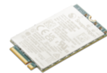
ThinkPad Foxconn SDX61 5G Sub6 PCIe M.2 3052 WWAN module for P14s G7 Intel
